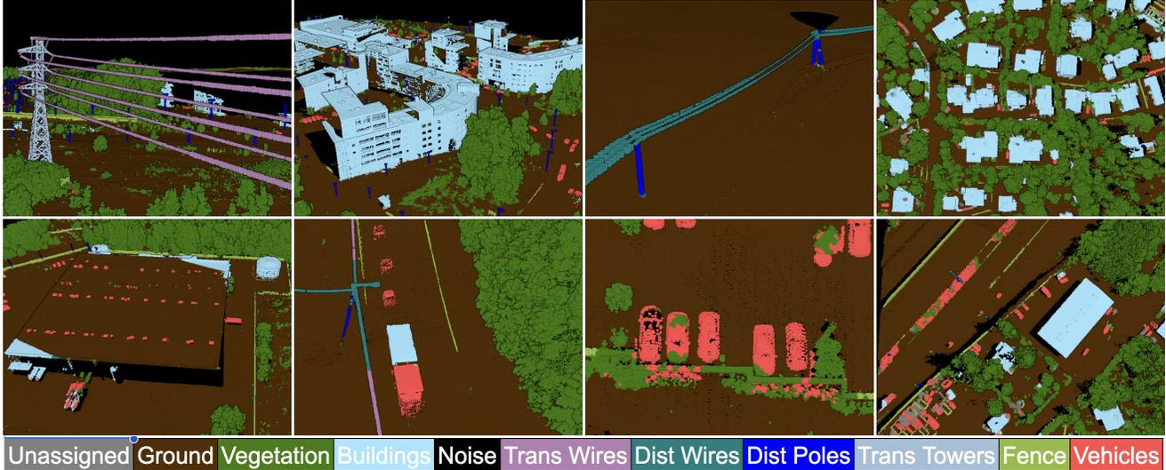
Figure 7. **Qualitative results of the best model.** We assess segmentation performance of the strongest baseline model on the test split of the proposed ECLAIR dataset. The top row demonstrates successful cases where the model performs well. In contrast, the bottom row highlights failure scenarios where the model produces noisy, inaccurate predictions.
