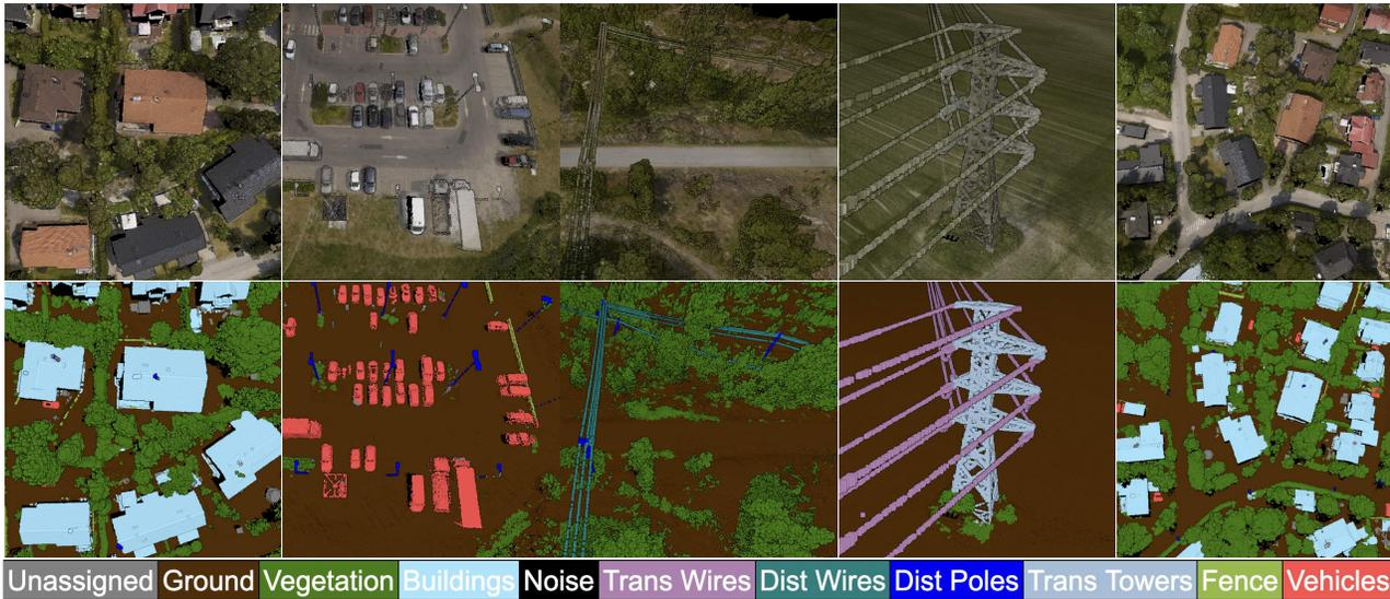
Figure 1. **Overview of the proposed ECLAIR dataset.** We introduce ECLAIR, a new outdoor large-scale aerial LiDAR dataset. It covers a total area of more than 10 square kilometers encompassing 11 semantic classes. The long-tail accurate annotations enable fine-grained semantic understanding. Different semantic classes are labeled by different colors.
